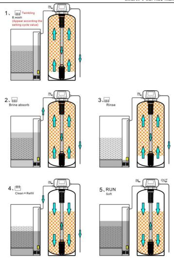
Pic7: GR-1 fixed bed back flow regenerate flow process
