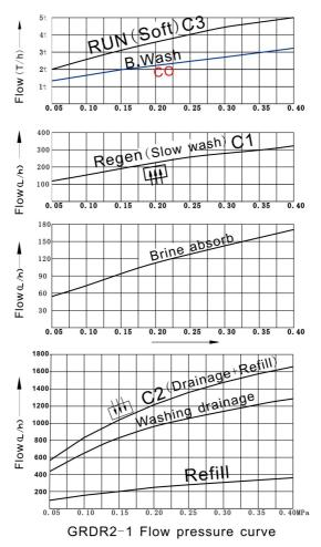
Pic14: GR2-1 /DR2-1 Curve of Flow and Pressure for the Valve
