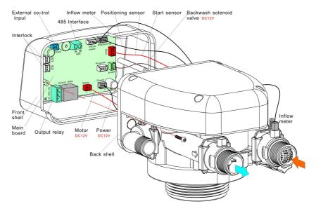
Pic18: Controller front shell disassembly(GRDR2-1\GRDR4-1)
