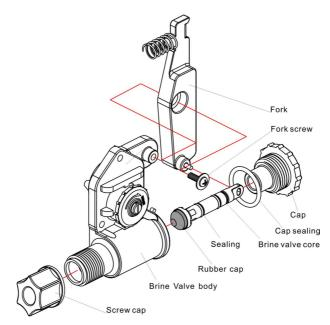
Pic22:Brine valve explode drawing (GR2-1 example)
