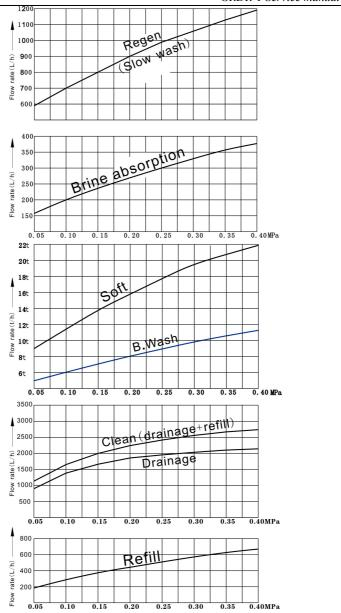
Pic16: GR10-1\GR10-1S Flow and Pressure curve
