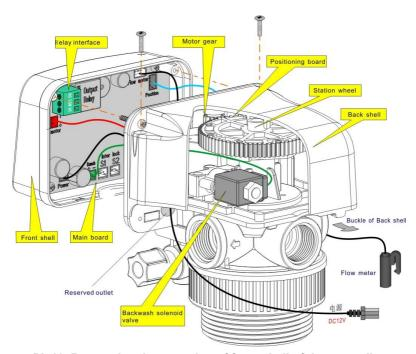
Pic11: Removal and connection of front shell of the controller
