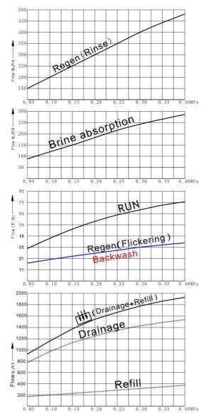
Pic13: GR4-2 Flow pressure curve
