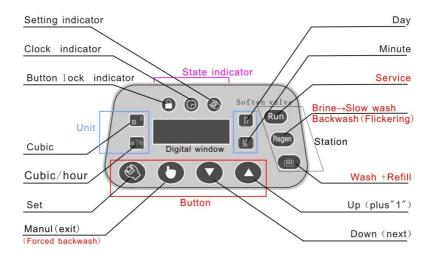
Pic1: Soften valve Controller interface
