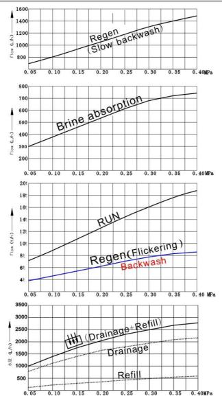
Pic14: GR10-2 Flow pressure curve
