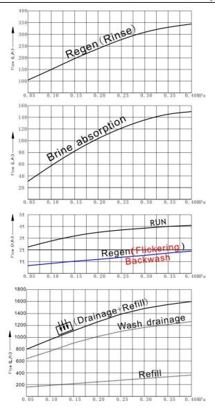
Pic12: GR2-2 Flow pressure curve
