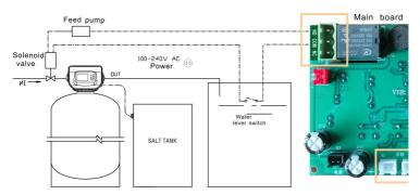
Pic3: Mode(b=00): Solenoid valve liquid level switch and feed pump.
