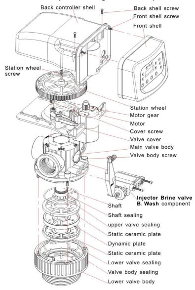
Pic15: GR-2 valve explode drawing (GR4-2 example)
